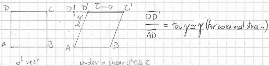
Hooke's law for elastic behaviour (linear relation between stress and strain) tells us that  $\gamma = \frac{1}{G}$  with  $G$  = shear modulus (or modulus of rigidity)
