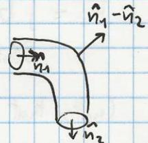
which tells us that  $\bar{F}^W$  is pushing the pipe diagonally, towards the outside of the elbow. Notice that the same happens if we invert the orientation of the flow.
